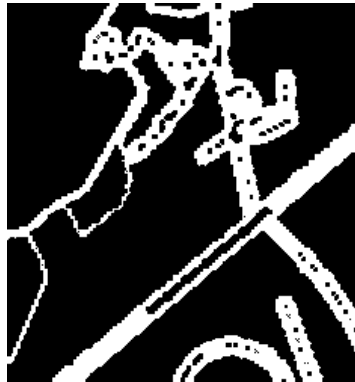
Figure (4.18): Merged image after removing one-pixel gaps.
